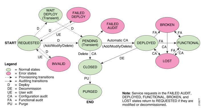
*Figure 11-3 Service Requests States Transition Diagram*
